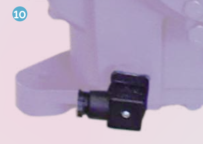
Oil sump heater
